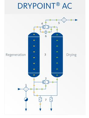
The cold-regenerated DRYPOINT<sup>®</sup> AC adsorption dryer ensures a continuous supply of high-quality air.
