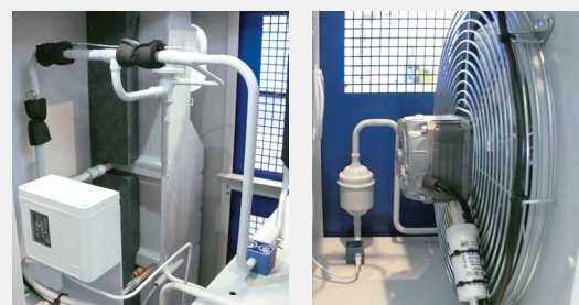
Internal view of a coated refrigeration dryer
