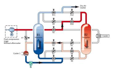
The whole procedure is executed with operating pressure, not only in the adsorption stage but also in the desorption and cooling stages. This therefore enables the resulting compression heat to be utilised for desorption for oil-free compressors for pressurised air.
