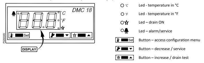
The DMC18 controls the alarms and the settings of the dryer operation and of the BEKOMAT drain.
