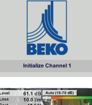
After the **METPOINT**<sup>®</sup> **CID** is switched on, it will be initialized and then switch to the leakage screen
