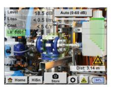
In order to automatically use the measured distance to calculate costs, you will need to enable the "Distance by Laser" option under "Parameter."
