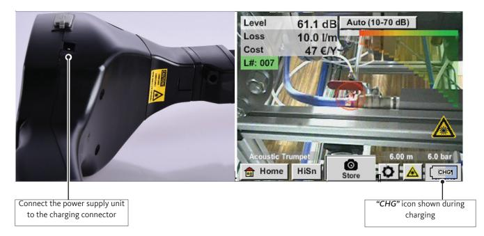
The **METPOINT<sup>®</sup> CID** will check the battery's state of charge and will start charging it automatically if necessary.
