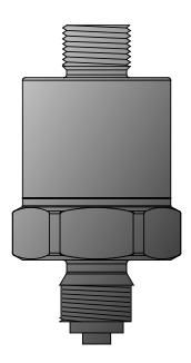
The **METPOINT**® pressure transducer of the PRM-SP series detects the relative pressure (gauge pressure) in **gaseous** and **liquid** media and transforms this measured value into a linear, pressure-proportional electrical output signal of 4 ... 20 mA or 0 ... 10 V.
