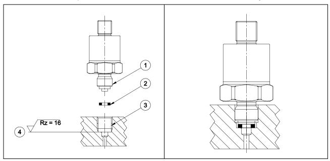
In order to seal the process connection (1) with a cylindrical thread (3) at the sealing surface (4), flat gaskets (2) are employed.
