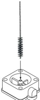
A technical drawing of a square membrane cover with a central circular opening. A long, thin cleaning brush with bristles is shown vertically, with its tip pointing into the central opening. A dashed line indicates the brush's path.                               | 5. Membrandeckel mit einer Reinigungsbürste Ø max. = 1,5 mm (0.05") reinigen.                         |
