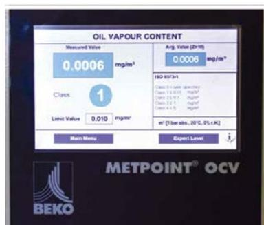
The METPOINT OCV monitoring system monitors the purity of the compressed air and certifies
