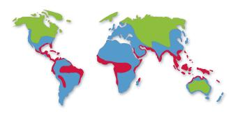
Depending on the climate and temperature, differing amounts of condensate can form. For the BEKOMAT® models, we therefore quote the performance values based on three climate zones.
