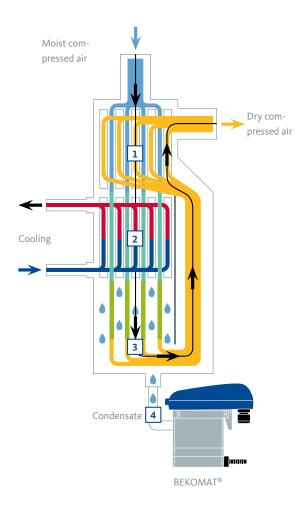
In the DRYPOINT<sup>®</sup> RA eco refrigeration dryer, the air is dried via a counter-flow process with optimised heat exchange (Counter-Flow) along the entire process path, the air flows in a constant downwards aligned direction without diversions.
