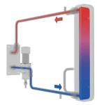
The water cooled plate heat exchanger (WC) is available for the following models from the DRYPOINT<sup>®</sup> RA/RS HP series:
