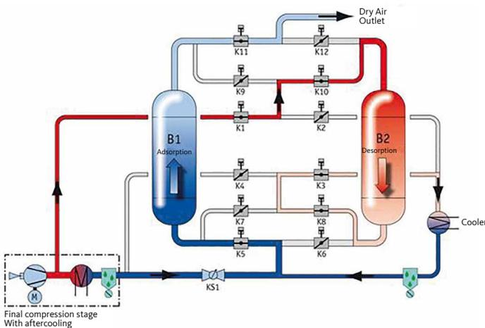
The whole procedure is executed with operating pressure, not only in the adsorption stage but also in the desorption and cooling stages. This therefore enables the resulting compression heat to be utilised for desorption for oil-free compressors for pressurised air.
