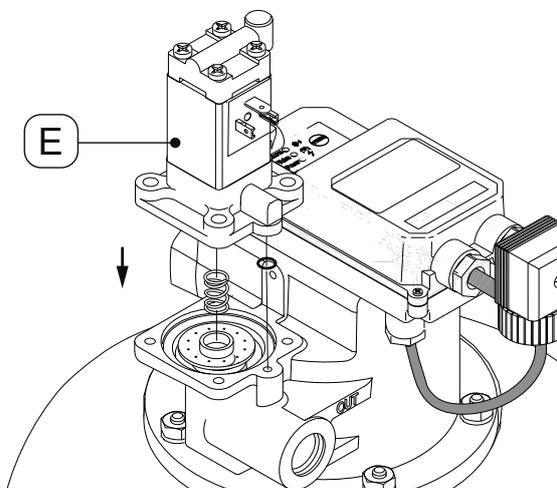
13. Place the valve unit **[E]** back on the membrane cap.
