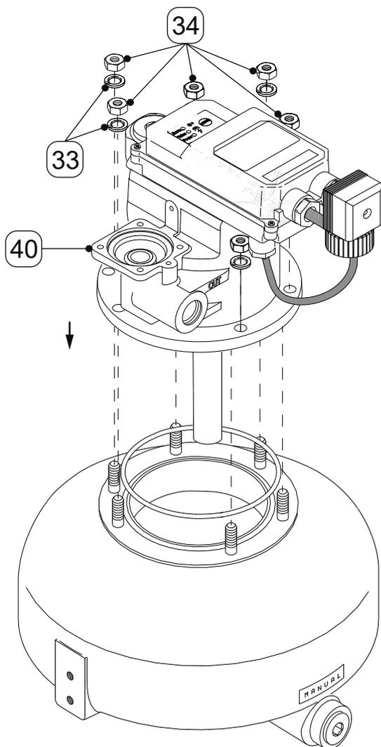
9. Set the housing upper part **[40]** in place again and screw tight using the nuts **[34]** and spring washers **[33]**.
