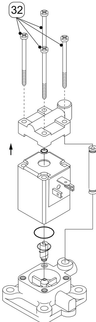
5. Loosen the screws [32] and take the valve unit apart.
