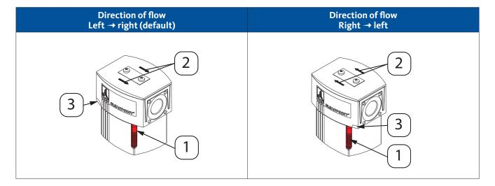
The housing head and the housing body are equipped with a double-start trapezoidal thread. The direction of flow through the filter can be adapted to the direction of flow in the pipe by turning the housing head through 180°. The direction of flow is indicated by arrows [2] and a raised marking [3] on the housing head. These must be aligned as shown. The safety slide [1] must always be in an easily accessible position on the front.
