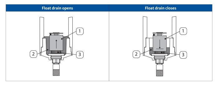
Both types of float drain are delivered with the position "Automatic discharge" from the factory. The knurled screw is screwed downwards as far as it will go.
