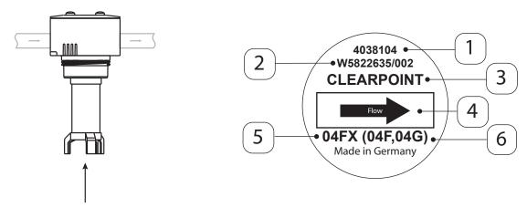
Adhesive label on the base of the filter element
