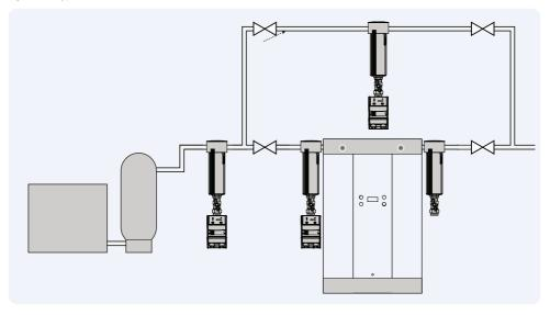
To prevent back flow into the dryer a non-return valve should be placed in-line, downstream of the dryer. This is essential when more than one dryer is used in a single application.
