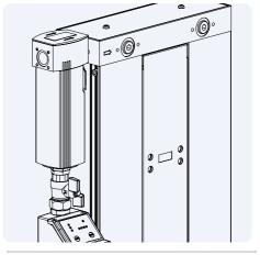
Figure 3.4: Connecting filter drain
