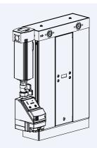
Connecting the pre-filter to the dryer
