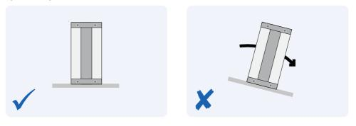
Figure 3.8: Drainage (all tubing should be secured up to the point of drain to prevent whipping during discharge)
