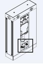
Figure 6.11: Diaphragm changeout stage 2
