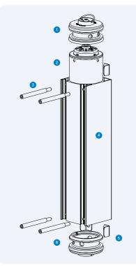
Fig 10.6 Top tower plug assembly
