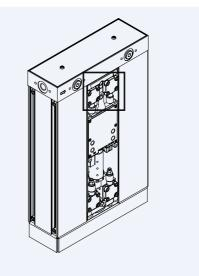
Figure 6.8: Purge plug changeout stage 2
