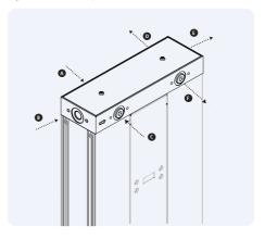
Figure 3.6: Reconfiguration of inlet/outlet ports
