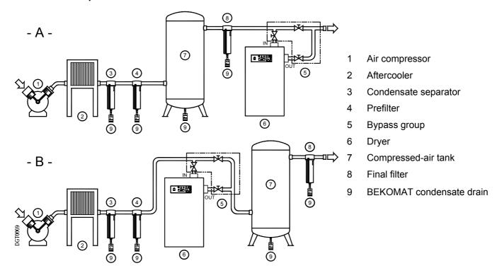
Installation  $type\ A$  is recommended when when the total consumption corresponds to the throughput rate of the compressor.
