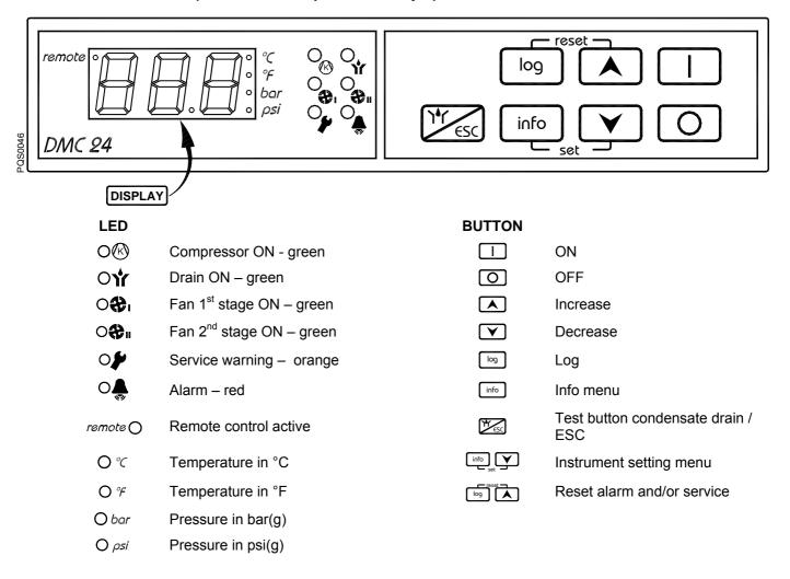
The DMC24 controls all operations, alarms and instrument settings of the dryer. The display and the LEDs indicate all operating conditions.
