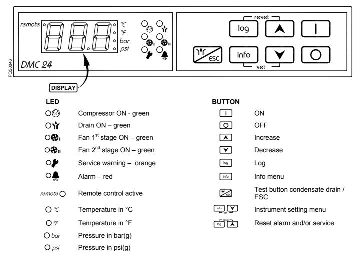
The DMC24 controls all operations, alarms and instrument settings of the dryer. The display and the LEDs indicate all operating conditions.
