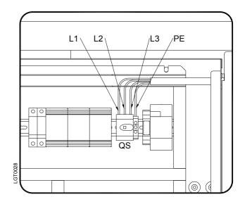
A residual-current device (RCD) with I∆n =0.03A is suggested. The cross-section of the power supply cables must correspond to the consumption of the dryer. In this respect, the ambient temperature, the cable laying conditions, the length of the cables and the requirements of the local electricity supplier need to be considered.
