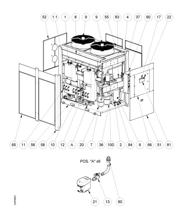
13.2.3 Exploded diagram DRYPOINT RA 10800-13200 water-cooled 1/2
