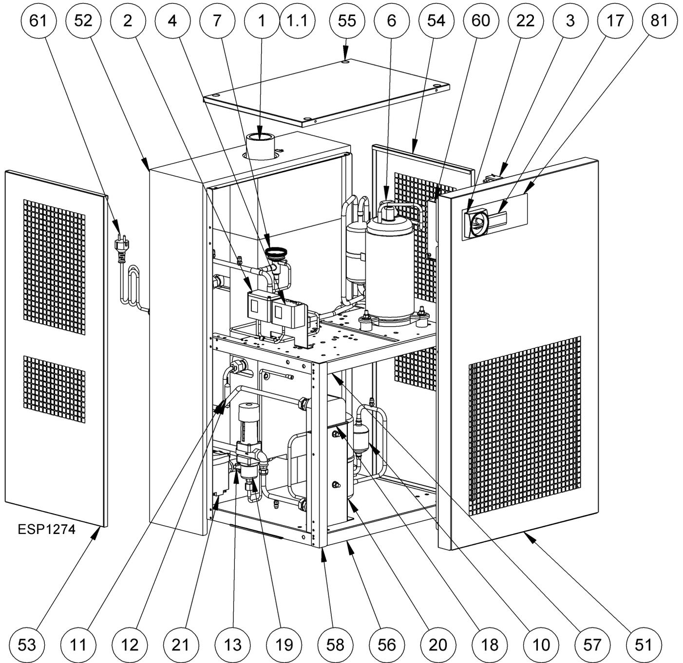
13.2.11 Exploded diagram DRYPOINT RA 750-960 Water Cooled
