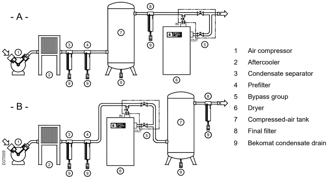
Installation **type A** is recommended when the total consumption corresponds to the throughput rate of the compressor.
