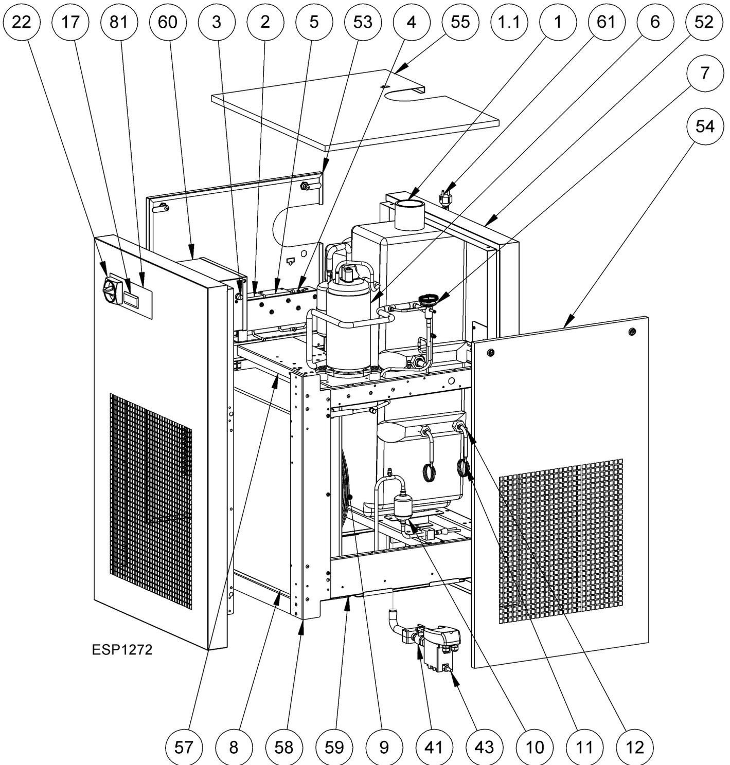
13.2.9 Exploded diagram DRYPOINT RA 330-370 Water Cooled
