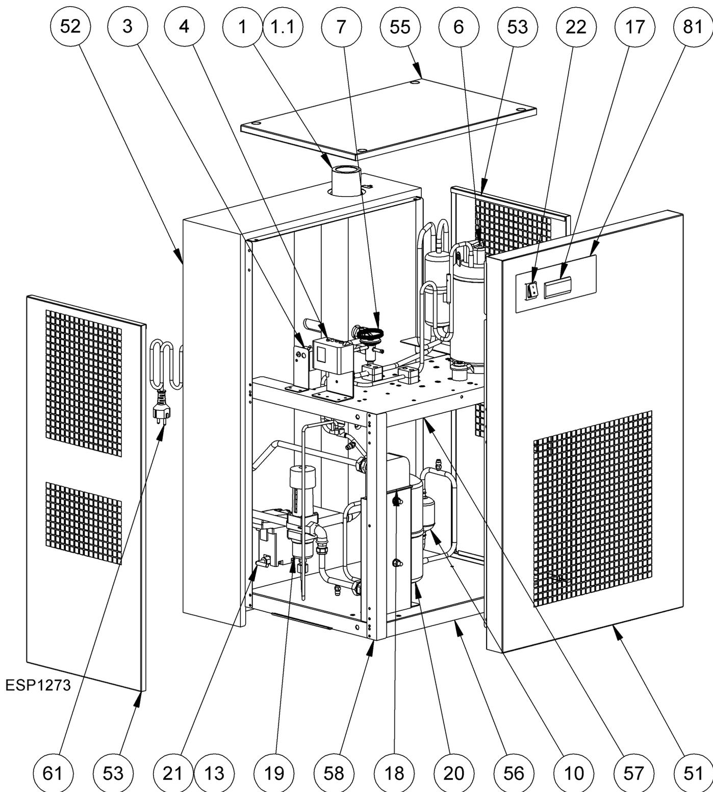
13.2.10 Exploded diagram DRYPOINT RA 490-630 Water Cooled
