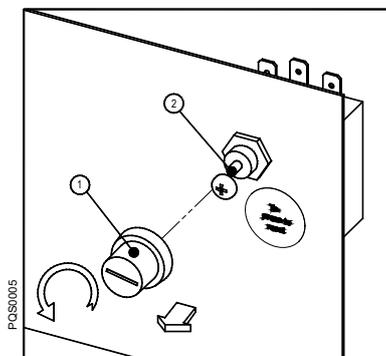
To ensure the operational safety and the soundness of the dryer, a safety temperature switch (TS) is installed at the refrigeration cycle. In the event that the pressure gas temperature is too high, the sensor of the temperature switch will stop the refrigerating compressor to prevent the pressure gas temperature getting too high.
