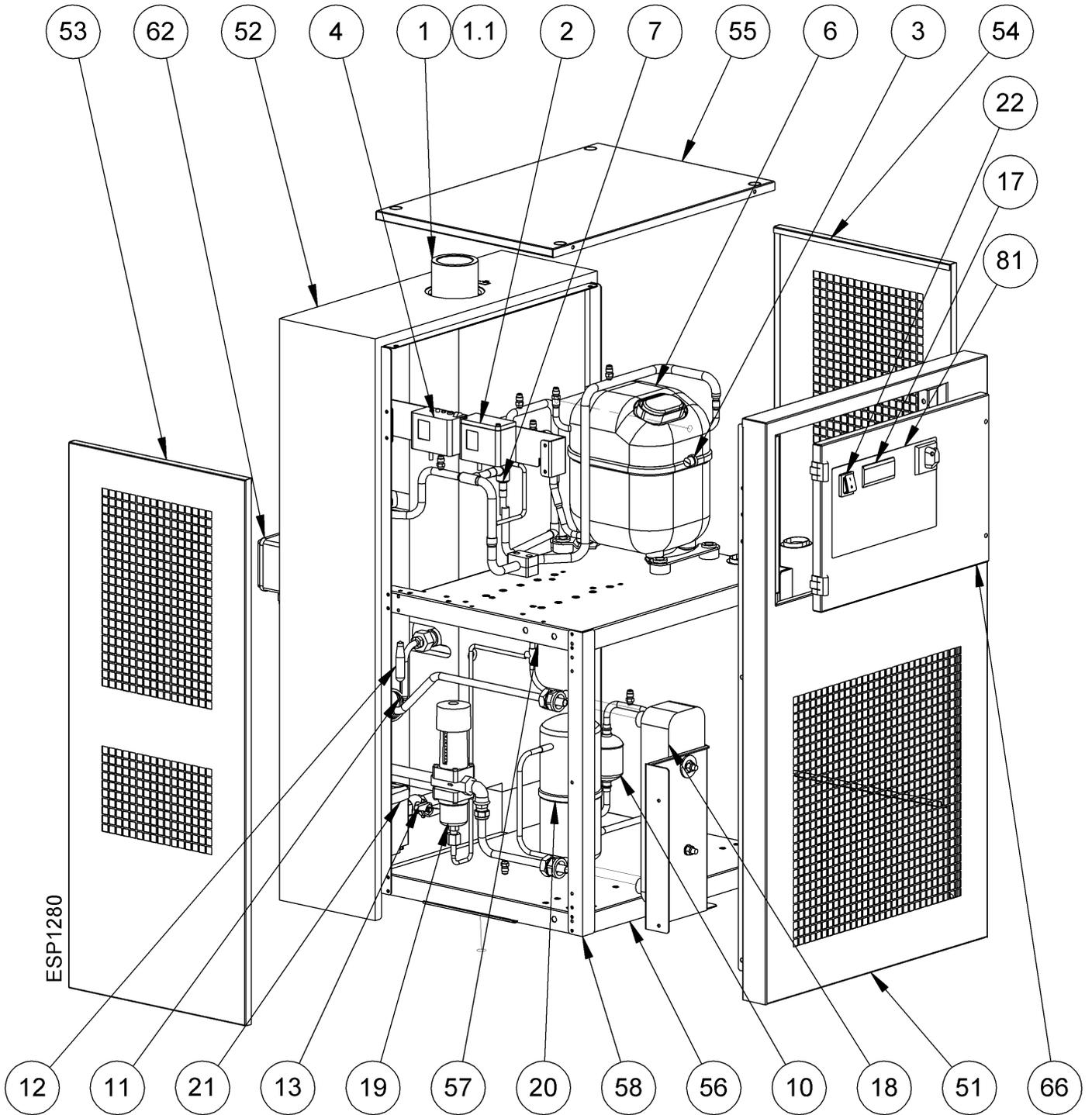
13.2.17 Exploded diagram DRYPOINT RA 750-960 3phase Water Cooled
