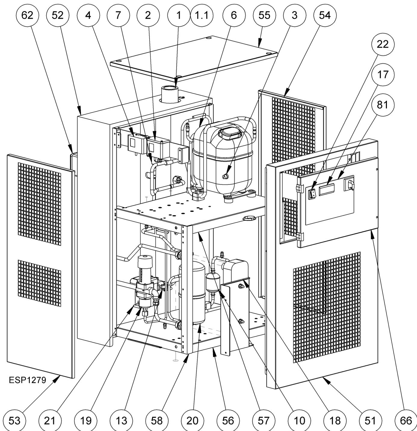
13.2.16 Exploded diagram DRYPOINT RA 490-630 3phase Water Cooled
