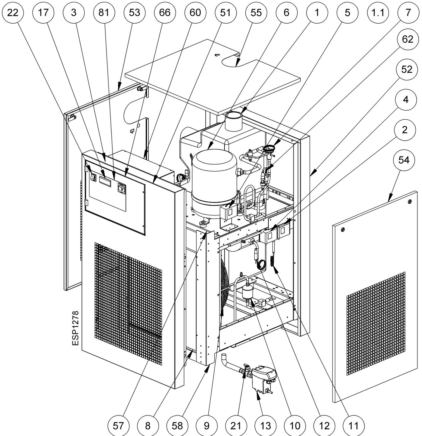
13.2.15 Exploded diagram DRYPOINT RA 330-370 3phase Water Cooled
