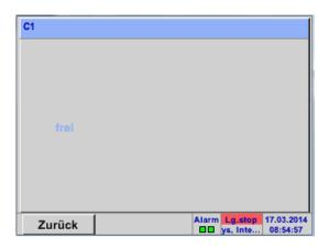
When *returning* from *Type* **no sensor** to sensor settings, the channel is displayed as *free*.
