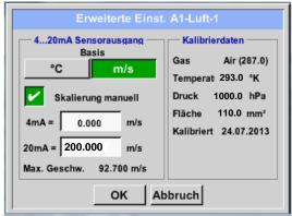
In the *advanced settings*, it can be determined whether the 4-20 mA analogue output of the sensor should be based on the flow volume or on the velocity.
