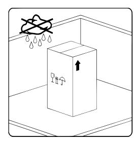
Store the METPOINT® BDL portable in its original packaging in a closed, dry, and frost-protected room. The ambient temperatures must not exceed/underrun the values indicated on the type plate.
