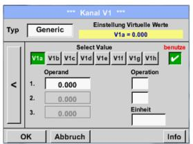
By pressing the 1st operand field, you will go to a selection list with the available hardware channels, virtual channels, and constant values.
