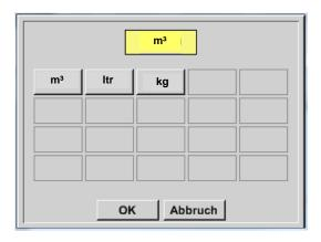
The available units for the unit of the *counter* for the *type* **pulse**
