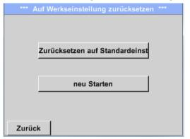
If required, the METPOINT® BDL portable can be re-booted by pressing the *Restart*-button.
