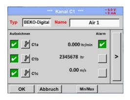
Subsequent to marking and confirming by *OK*, the configuration of the sensor is completed.
