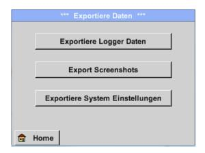
With Export logger data and Export system settings, the recorded measuring data and the stored settings can be transmitted to a USB stick.
