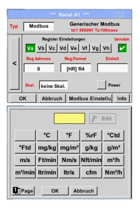
Pressing the *Unit* text field will lead you to a list with the available units.
