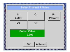
By pressing a hardware or virtual channel button, e.g. *11*, a selection list will open, showing the measuring channels or measured values that are available per channel, including defined virtual channels.
