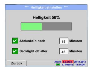
Here, the desired *brightness* (15 ... 100%) of the display can directly be set.
