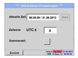
By pressing the *Time zone* text field and entry of the correct *UTC*, the correct time can be set worldwide.
