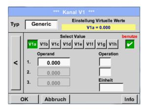
A virtual value is activated by pressing the respective *Value button*, for example *V1a* with subsequent actuation of the *Use button*.
