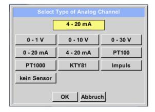
Selection of the required sensor type by pressing the respective button, here, for example 4-20 mA.
