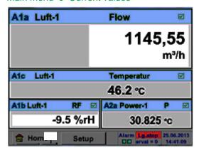
The *current values* view allows for the indication of 1 to 5 freely selectable measured values.
