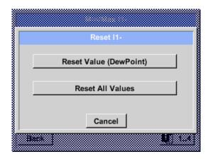
It is possible to reset an individual measured value such as the pressure dew point here, or all of the *min. and max.* values of the sensor, if required.
