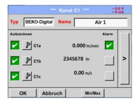
With the *recording* buttons, the measuring data are selected which will be stored at an **activated data logger**.
