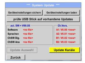
When, after having pressed the *Check USB* stick for available updates button, the following messages (no file) appear in the window, the METPOINT® BDL portable is not correctly connected with the USB stick or no data are available.
