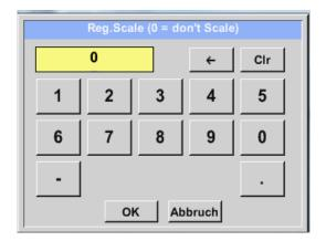
The application of this factor allows for the adjustment of the output value by the latter.
