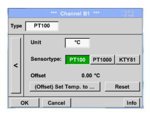
Here, the sensor type *PT100* and the *unit* °C were chosen. Alternatively, the sensor types *PT1000* and *KTY81*, as well as the *unit* °F can be selected.
