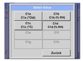
By pressing the desired channel button, e.g. *C1b*, the selection is accepted.
