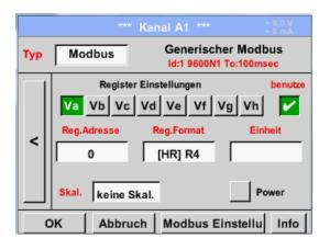
Via Modbus, up to eight registry values (from input or holding registers) of the sensor can be read out.
