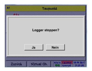
If the data logger is activated, the following window appears. By pressing *yes*, the data logger can be deactivated.
