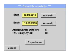
By means of the *Selection* buttons, a period of time between *start* and *end* can be set. The stored bitmaps, which are within this period, are exported.
