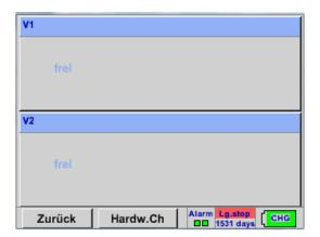
After having activated the "virtual channels" button in the sensor setting menu, an overview of the available four channels will appear.
