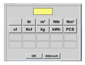
For the *unit* **pulse**, a flow volume or energy consumption can be chosen as a unit.
