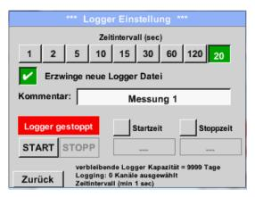
By pressing the *Force new logger-file* button, a new recording file is created, and with the selection of the *Comment* text field, a name or comment can be entered.
