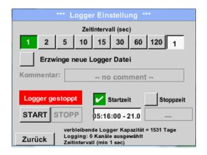
In the uppermost row, the pre-defined *time intervals* 1, 2, 5, 10, 15, 30, 60, and 120 seconds can be chosen for the recording.
