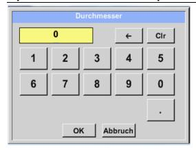
Here, the *Inner diameter* of the flow pipe can be entered in the event that it was not automatically correctly set.
