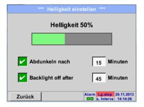
By means of the *Darken-after* button, the *brightness* can be reduced to a minimum at the end of a time interval to be defined (here after 15 minutes), or completely switched off.
