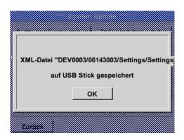
Stores the *channel and system settings* in an XML format on a USB stick.
