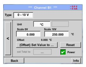
With the *Set-value-to* button *(offset)*, the measured data of the sensor can be set to a certain value.
