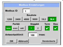
The corresponding Modbus ID can be taken from the data sheet of the sensor (here, for example, 1).
