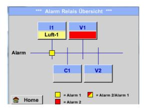
In the *alarm overview*, you can immediately see whether the alarm is an *alarm-1* or an *alarm-2*.
