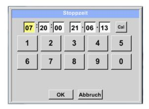
After having pressed the *Date/time text field*, the input window will appear, in which the zone of the time or date which is highlighted in yellow can always be set or changed.
