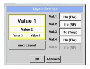
Here, the desired layout can be selected by pressing the *Next Layout* button.
