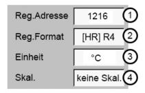
The entry of the Modbus parameters is implemented via the white buttons (1) - (4).
