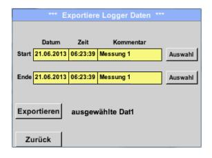
By means of the *Selection* buttons, a period between *start* and *end* can be set. Stored measured data within this period are exported.
