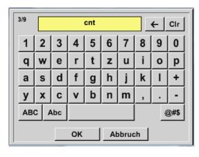
Define the unit and accept with OK. By means of buttons ← and *Clr*, the entry can be corrected. Button ← erases the last character Button Clr erases the entire value
