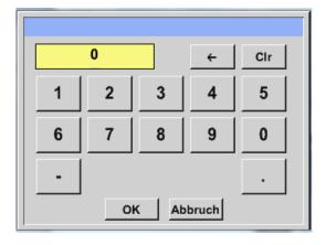
If the *Const. value* button was pressed, the value needs to be determined via the numeric keypad. By pressing the *OK* button, the value is accepted.
