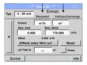
Selection of the units by pressing the respective unit, **Measured value** or **Consumption rate** text fields.
