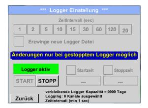
The data logger can also be activated and deactivated without activated time settings, namely by means of the *Start* and *Stop buttons*.
