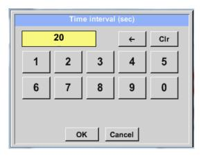
A deviating individual *time interval* can be entered into the text field with the white background on the upper right where the currently set *time interval* is always indicated (here, for example, 20 seconds).
