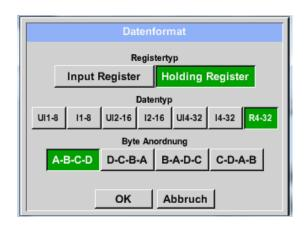
By means of the *input register* and *holding register* buttons, the respective Modbus register type is selected.
