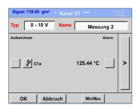
Scaling of the sensor (here, for example, *type* 0-10~V - corresponds to  $0-250^{\circ}C$ ) can be found in the data sheet of the connected sensor.
