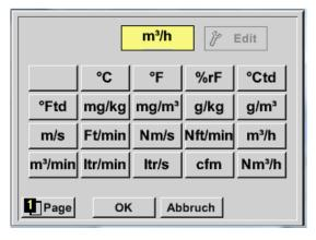
The selection of the unit is implemented by pressing the desired unit button. The unit is accepted by pressing the *OK* button.
