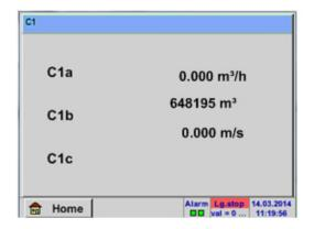
The *Channels* view shows the current measured values of the connected sensor. In the event that the adjusted alarm limits are exceeded or underrun, the respective measured value flashes yellow (*alarm-1*) or red (*alarm-2*).
