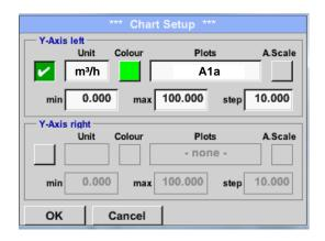
Now, the y-axis scaling with *min*, *max*, and *grid* can be set.
