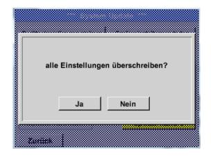
By means of the *Loading device settings* button, the channel and system settings can be reset to the status of when it was last saved.
