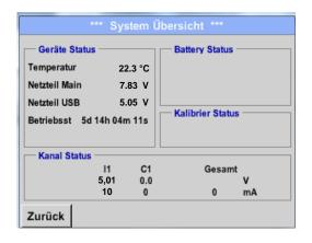
The *system overview* menu item provides information on the applied voltages and currents of the individual and the entire *channels*, as well as on the voltage supply of the *power supply units*.
