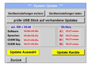
When the METPOINT® BDL portable is correctly connected with the USB stick and newer versions are found, these are indicated.
