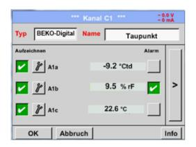
The METPOINT® BDL portable recognizes whether the connected sensor is a flow rate or a dew point sensor from BEKO TECHNOLOGIES GMBH and automatically sets the **BEKO** subtype correctly.
