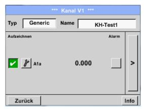
With the *Recording* buttons, the measuring data are selected which are stored at an **activated** data logger.
