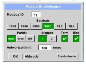
Here the *Modbus ID* is entered which is determined for the sensor, permissible values are 1 - 247, (ex. here *Modbus ID* = 12)
