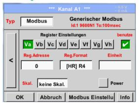
The sensor provides the measured values in registers. The values can be located and read out by the METPOINT® BDL PORTABLE via Modbus.
