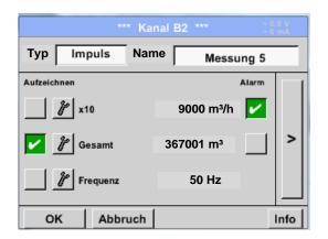
Normally, the numerical value with the unit stands for **1** pulse on the sensor and can directly be entered into the **1** pulse = text field.
