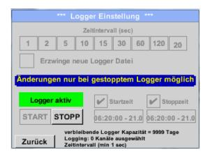
Subsequent to the *start* or *stop time* activation and the implemented settings, the *Start* button is pressed and the data logger is on *active*.
