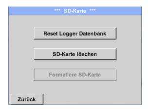
By pressing the *Reset logger data base*, the currently stored data are blocked from use in the BDL portable. However, the data remain stored on the SD card, and are available for external use.
