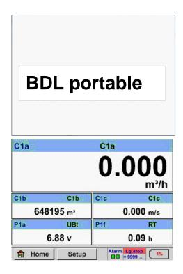
Subsequent to the switching-on of the METPOINT® BDL portable, the channel is initialised and the "*Current values*" menu appears.
