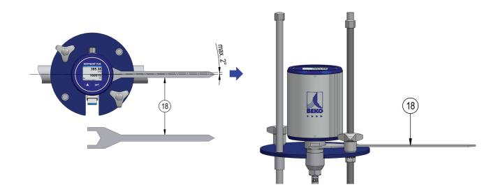
12. After the operating position of the sensor has been reached, fix the upper bracket [4] with the locking bolts [9] and the positioning handles [7].
