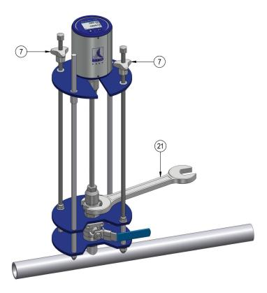
6. Further unscrew the loosened mass flow meter METPOINT® FLM SF53 and thereby carefully guide it upwards together with the upper bracket [4] until the FLM SF53 is completely screwed out of the ball valve [1] and can be removed to the front from the cut-out of the upper bracket [4].
