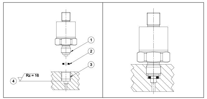
In order to seal the process connection (1) with a cylindrical thread (3) at the sealing surface (4), flat gaskets (2) are employed.
