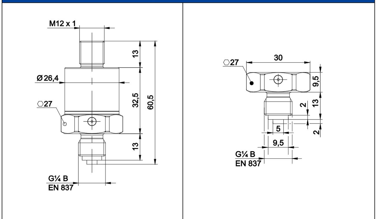
Connection adapter, R $\frac{1}{4}$  and  $\frac{1}{4}$  NPT, width A/F (German "Schlüsselweite") 27
