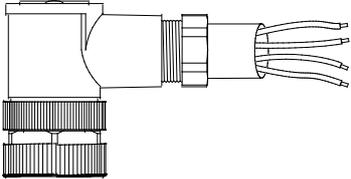
A technical drawing of an M12 angle connector. It features a 90-degree elbow with a threaded end on one side and a cable end on the other. The cable has four individual conductors protruding from a common sheath. | 4025252      |
