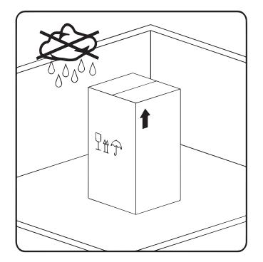
To store the device, place it in its original packaging and store it in an enclosed, dry and frost-free room. Ensure that the storage temperature does not exceed the limits specified on the type plate.
