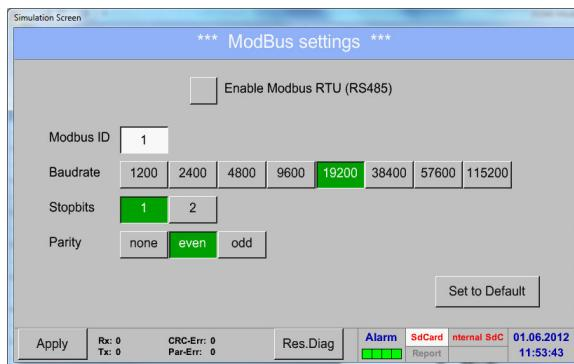
By communication via Modbus TCP the **Modbus Id** have to be set only and confirmed by pressing **Apply** button.
