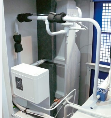
Inside of coated refrigeration dryer
