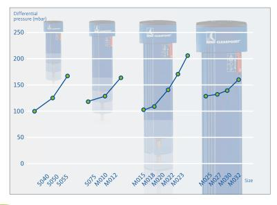
The differential pressure for the new S-Filter in wet-saturated condition for the modular constructed filter dimensions with energy-efficient designed volume flow. The jumps in the curve result from the respective lengths / diameter relationships fir the various filter sizes.
