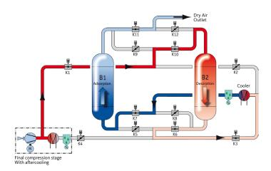
The whole procedure is executed with operating pressure, not only in the adsorption stage but also in the desorption and cooling stages.
